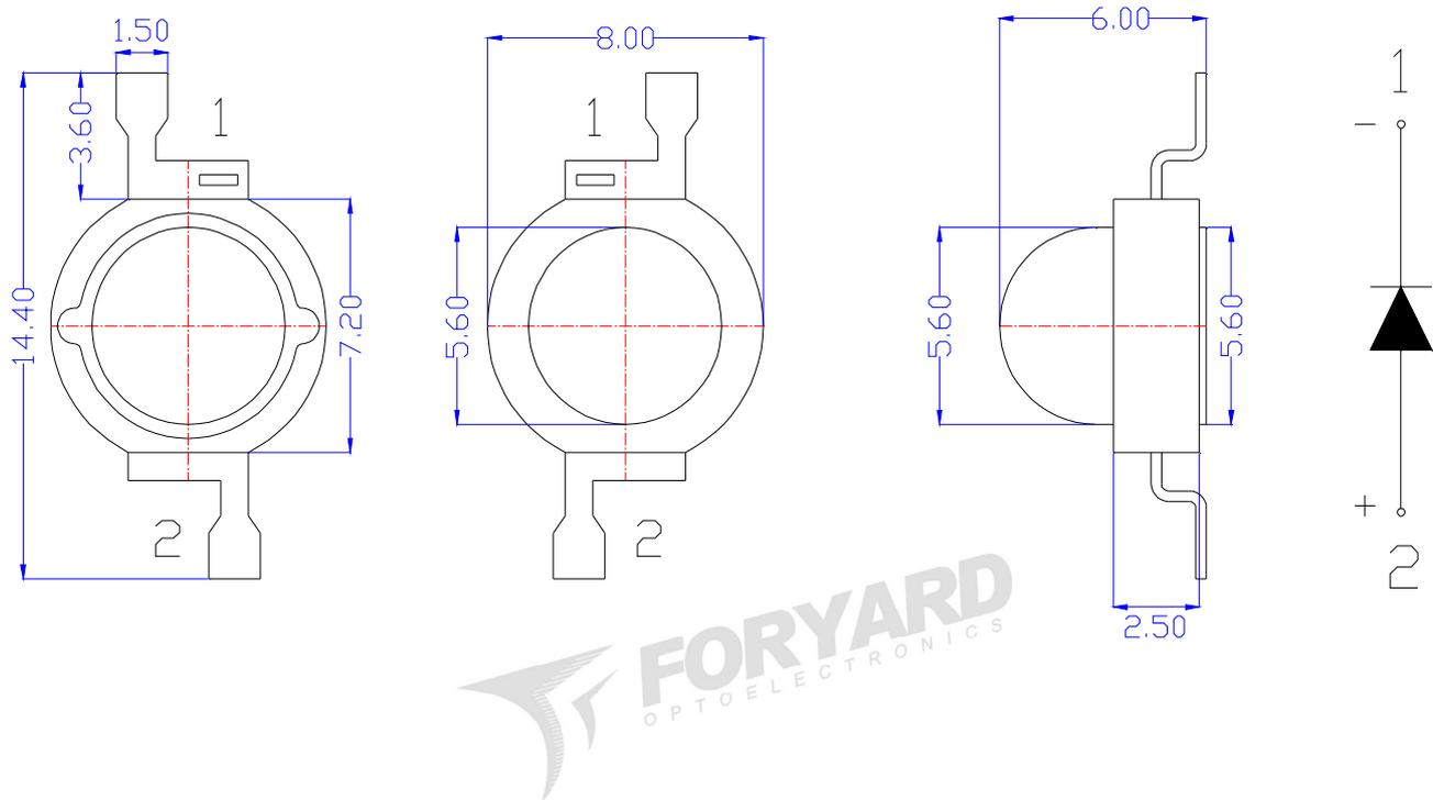
**■ Recommend Soldering pad design(unit=mm)**
