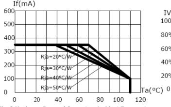
Fig. 3 Maximum Forward Current vs Ambient Temperature
