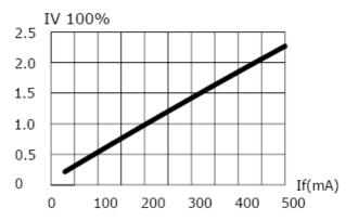
Fig. 2 Relative Luminous Intensity vs Forward Current
