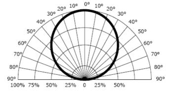
Fig. 6 Relative Luminous Flux vs Radiation Angle
