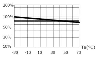
Fig. 5 Relative Luminous Flux vs Ambient Temperature
