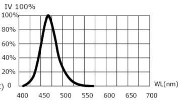
Fig. 4 Relative Luminous Flux vs Wavelength
