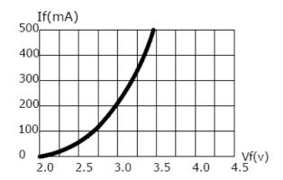
Fig. 1 Forward Current vs Forward Voltage
