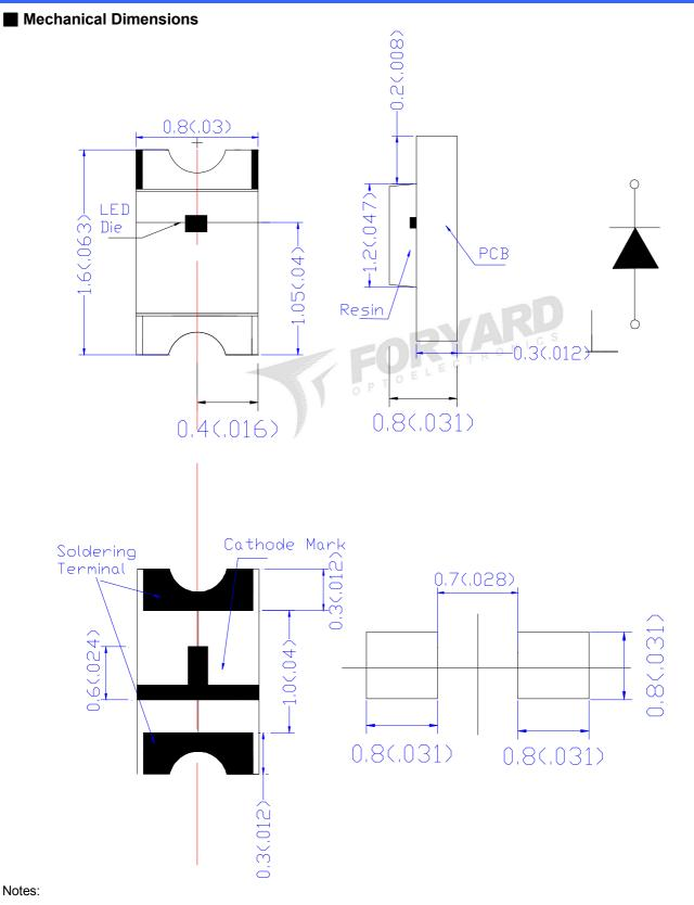
1. Dimension in millimeter [inch], tolerance is ±0.25 [.010].
